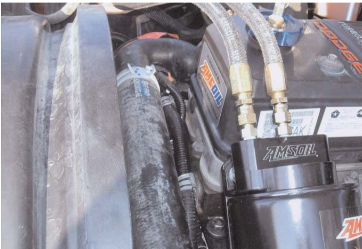
Custom-made bracket allows for use of the EaBP100 on this turbo-diesel pickup.
