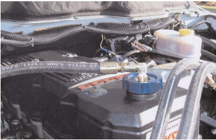
The valve cover cap is the by-pass return line.
