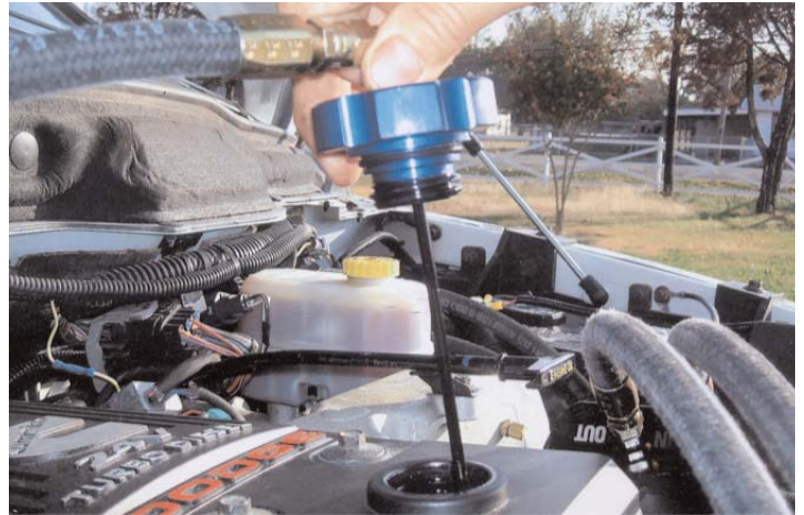
The engine is running and everything is flowing properly as indicated by the stream of oil.
